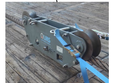
Calibrated line running tensioner used on vessel wire.
