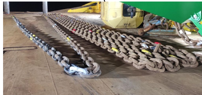
Colour coding of chain links to enable measurement distance, and if required, depth of anchor chain.
