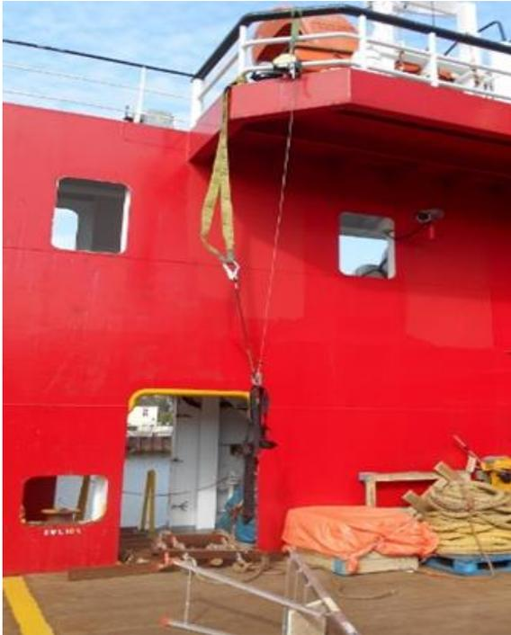
Incident location, with harness hanging from belt, and fall arrestor connected for retrieval, as a demonstration of the situation at the time of the incident. The fallen ladder was part of the drill scenario.
