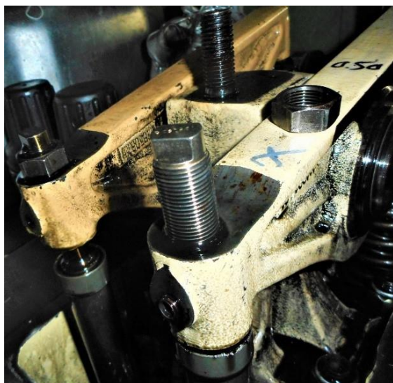
Picture showing rocker arm adjusting screw with locking nut removed / dismantled
