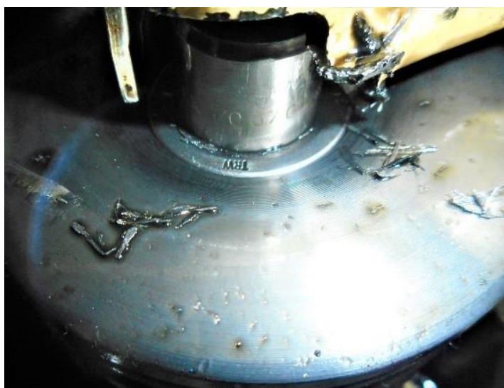
Picture showing partial destruction of the exhaust valve tappet tip, showing also the valve roto cap.
