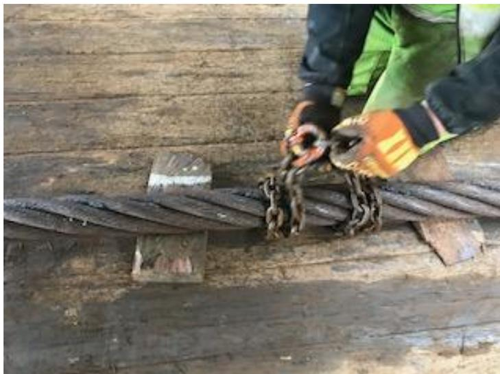
Picture 2 – Disconnection of the chain (post-incident solution)
