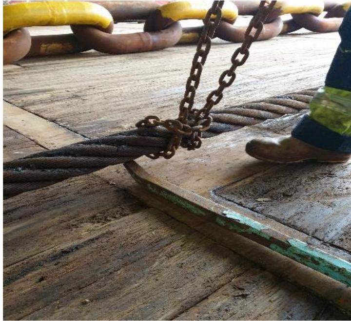
Picture 1 – Crow bar used to support the tow wire
