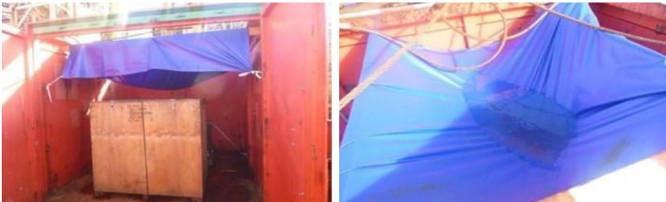
The above photo shows an open top CCU delivered offshore with a tarpaulin & baton cover.
