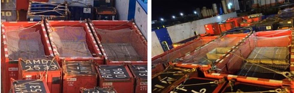
The above photo taken during the trial shows 3 x open top CCU's backloaded on the PSV's deck. Note that the lifting gear cannot fall inside the CCU's and snag on the cargo, yet wooden batons are not being used to support the net covers.
