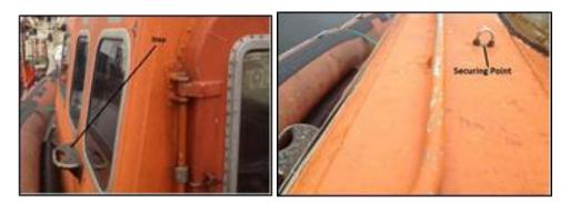
Once in position at the aft end of the DC the Boatman climbed up onto the step to receive the 'O' ring but did not secured his harness to the securing point on top of the DC.
