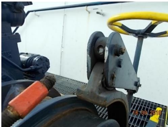
03a – Failed section of brake assembly
