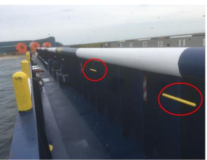
Photos 2 & 3; Additional snag hazards identified on other vessels
