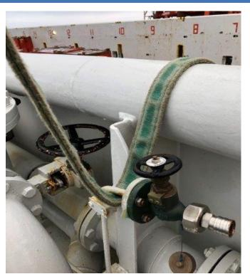
**Photo 1;** Simulation of the hang-off strop caught around the air valve
