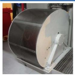
Following the incident, a protective frame was built around the tugger winch to prevent a similar incident from happening again.
