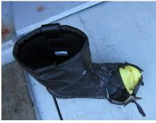
As the winch barrel rotated the wire securing bar trapped the AB's foot between the winch support plate and the rotating barrel crushing his foot as it rotated.
