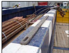
Three foot flat bar weighing approximately 4 kg found on top of 20' half height whilst it was back loaded to the vessel.
