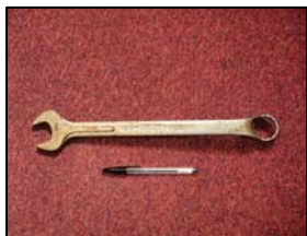
30 mm Ring Spanner left on a tank that was being back loaded to the vessel.
