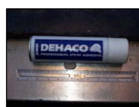
Aerosol left on horizontal beam of a tank back loaded to the vessel, as it landed on deck the can fell off.
